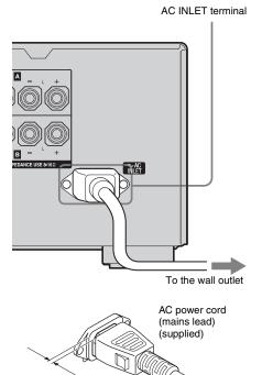
A several space is left between the plug and the rear panel even when the power cord (mains lead) is inserted firmly. The cord is supposed be connected this way. This is not malfunction.
